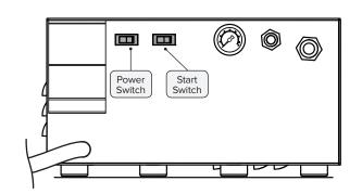
**CAUTION:** Do not operate misting pump without filter. **CAUTION:** Do not plug fan into outlet on misting pump.
