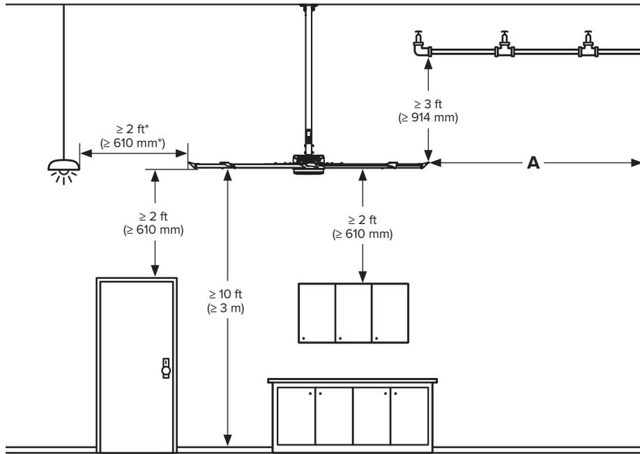
For the minimum clearance to combustibles, see the manufacturer's requirements.
